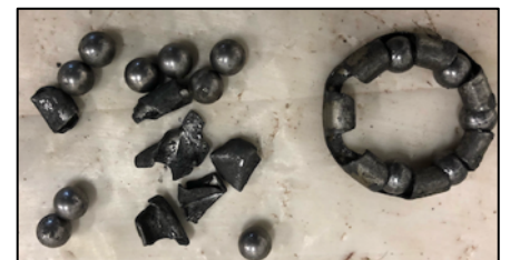
Bearings needing replacement
