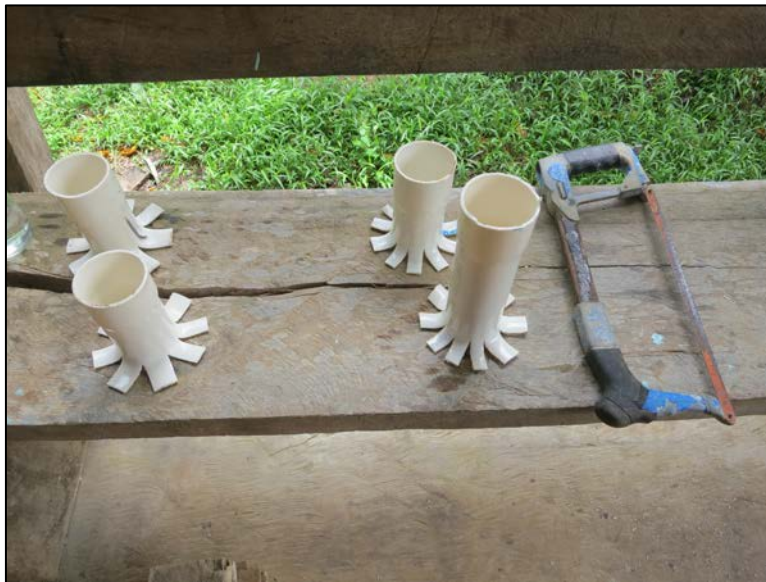
PVC pipes shaped and ready to use in making the tank lids
